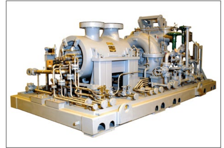
Figure 1: Elliott hydrogen hydrocracker compressor used in refinery processes. This unit processes a low mole weight gas (4.0 MOL) that is approximately 91.5% hydrogen. It has five impeller stages, an inlet pressure of 2,335 psia, maximum continuous operating speed of 12,027 rpm, and can process 1,692 ICFM through its 10-inch inlet nozzle.
